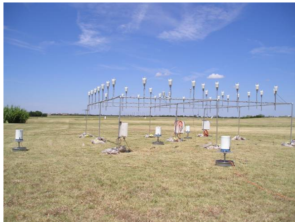
Figure 1. The Oklahoma City Urban Micronet Intercomparison Facility.
